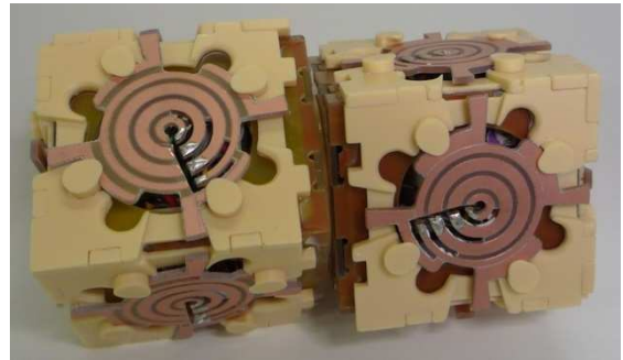
Fig 3. Rotational module. The left node contains the servo and the right node contains the electronic board.
