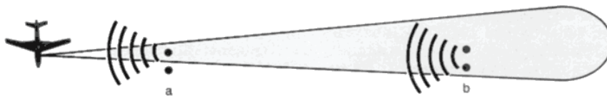
Figure 13.18: The cross range resolution degrades with range as shown. At position (a) the targets are resolved but at position (b) the targets, with the same spacing, are not resolved
