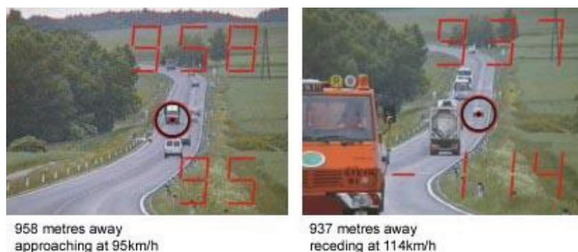
Figure 13.16: Effectiveness of narrow beam for measuring speed on congested roads
